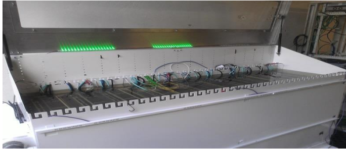
Oil-based cooling system
